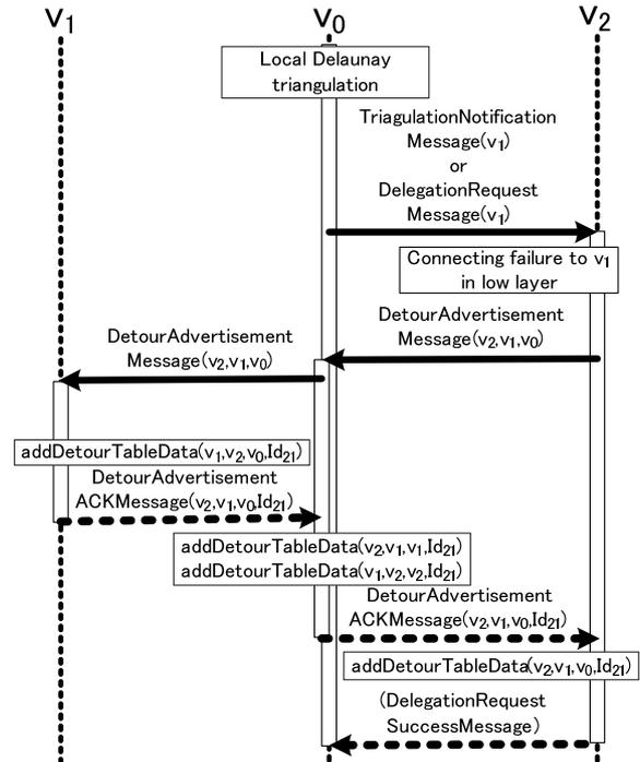
Fig. 10 Detour table construction sequence diagram.
