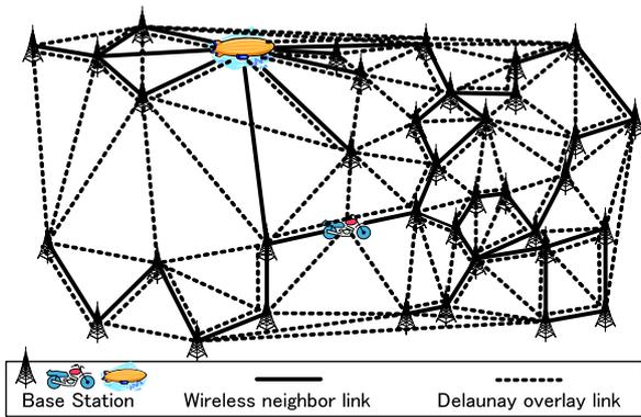
Fig. 2 Wireless mesh BSs and Delaunay overlay network.
