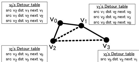
Fig. 11 Constructing nested detour paths ( $v_3-v_1-v_2$ ).
