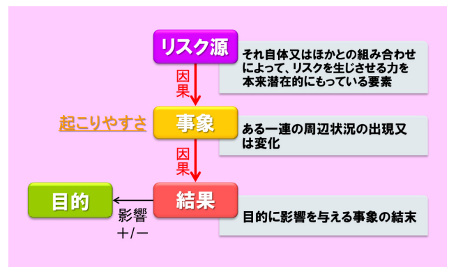
図 2 リスク表現におけるリスク源と事象と結果の関係 Fig. 2 Relationship among risk sources and their event and its consequence.
