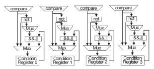
Fig. 9 Block diagram of parallel reconfigurable comparison module.
