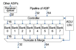
Fig. 8 Architecture of reconfigurable multi bank memory.
