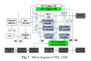
is used to calculate the address of elements in memory, detect access conflict and select available banks. LUT4\_Wb module reads data from memory banks and allocates data to the proper position in a register. If data fail to be accessed in one cycle, the rest of unavailable data will be accessed in the following cycles.
