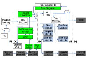
Fig. 11 Block diagram of 2D ASIP.
