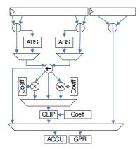
Fig. 15 Block diagram of post processing module.
