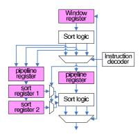
Fig. 14 Block diagram of sorting module.
