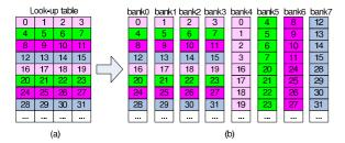
Fig. 4 (a) The content of look-up table. (b) The content after allocation in memory banks.
