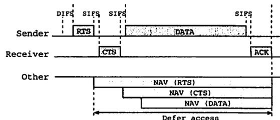
Figure 1: RTS/CTS access mechanism
