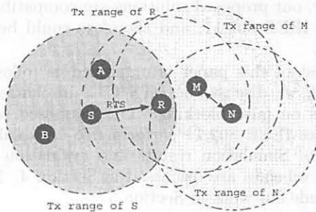
Figure 2: RTS/CTS induced false blocking. Node A and B is unnecessarily blocked by node S's RTS
