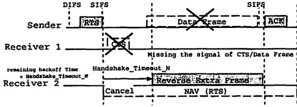
Figure 4: Reverse Extra Frame transmission
