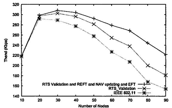
Figure 8:  $Th_{end}$  (number of connection 30 and offered load is fixed at 450 kbps).
