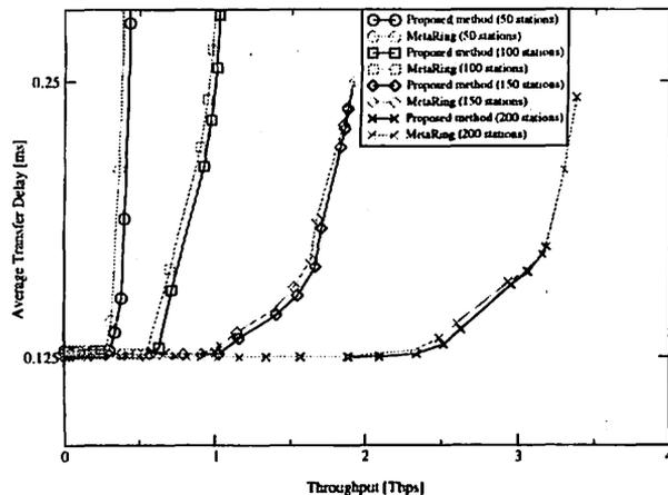
Figure 8: Performance characteristics for different number of stations.
