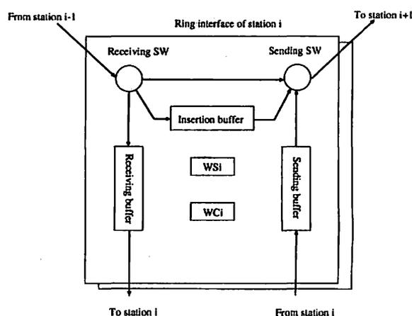
Figure 6: Ring interface structure.
