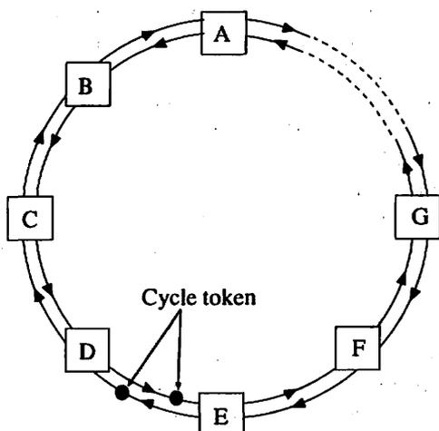
Figure 5: A bidirectional dual ring network.
