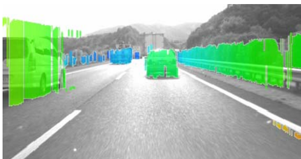
図7 短冊の視差の位置に棒として投影した結果 Figure 7 Projected image of the rectangles according to the obtained disparities
