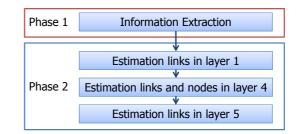
Fig. 2: Flow of the proposed method 1) all devices support SNMP; 2) there is no hub; 3) there is no Virtual Local Area Networks (VLANs); 4) the AFTs are complete.
