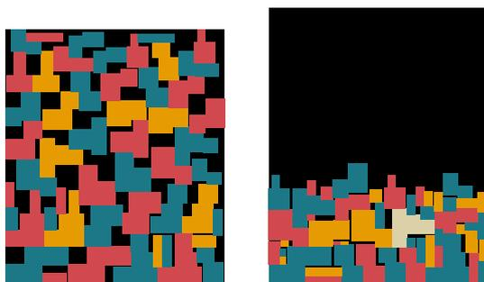
Fig. 3 Layouts when the algorithms pack half of the items (left: the bottom-left algorithm, right: the best-fit algorithm)
