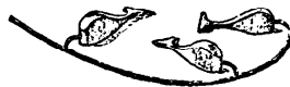
Splines are made of xylonite, and also of wood, with a groove along one edge in which the finger of the weight fits. The weights
