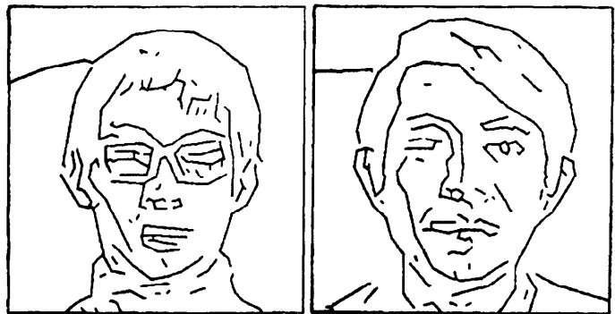
Fig. 12 Modified edge value with threshold setting ( K_s=6.0 , K_t=0.8 )
