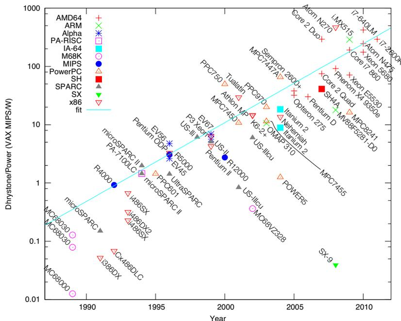
**Fig. 3** Dhrystone/power; Dhrystone performance divided by the power consumption in running state. Not all systems in Fig. 1 is on this figure.
