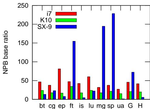
Fig. 5 NPB OpenMP results on Intel Core i7-860@2800 MHz (8T)/ICC, AMD Phenom 9350e@2000 MHz (4T)/GCC and NEC SX-9 (4T)/SXCC; G: Geometric mean, H: Harmonic mean
