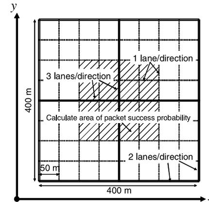
**Fig. 7** Simulation road model.
