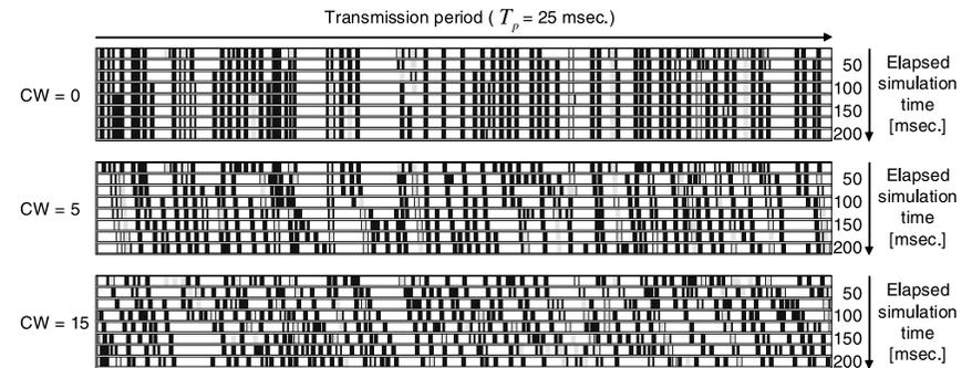
Fig. 10 Transmitted timing of DATA per transmission period ( $T_p = 25$  ms).
