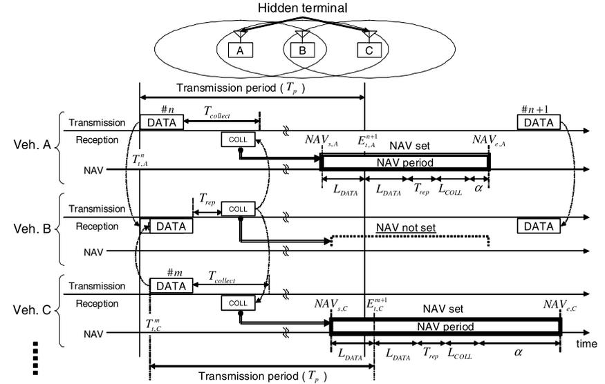
Fig. 3 Packet collision retrieval method in PB-TRMA.
