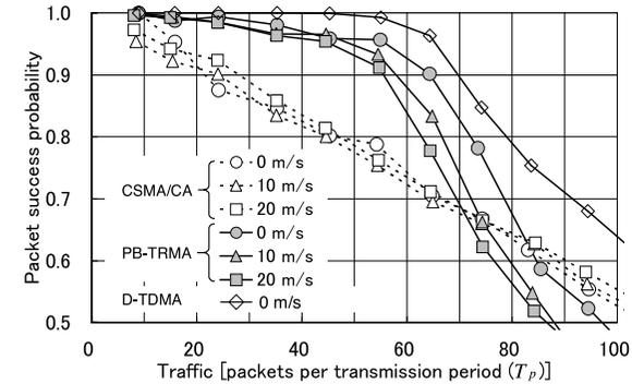
Fig. 17 Performances of PB-TRMA, D-TDMA and CSMA/CA.
