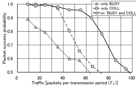
Fig. 13 Packet success probability for communication traffic in PB-TRMA.
