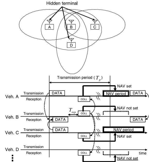
Fig. 5 Hidden terminal detection by receiving COLL.
