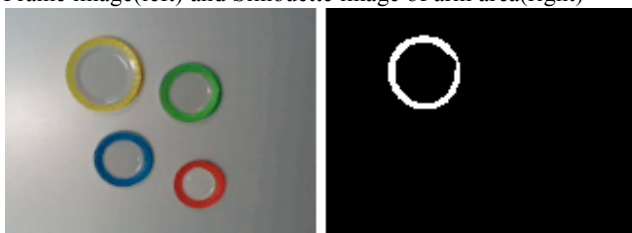
図5 FDT で使用する皿の例と皿の縁の色領域の抽出例(黄色) Fig5. The color is given to each edge of a plate (left) and Extraction of yellow plate (right)
