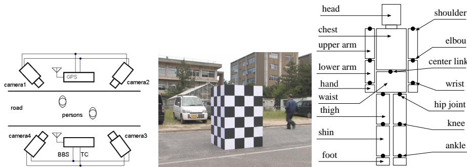
図 1 屋外多視点カメラの構成 (左), カメラ較正用物体 (中), 身体多関節モデル (右) Fig.1 Set up of synchronized cameras in outdoor (left), calibration box (center), and articulated body model (right).
