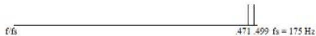
Figure 6 Difference in digital frequency between 82.4 Hz and 87.3 Hz if the sampling frequency is 175 Hz is .499 - .471 = .028
