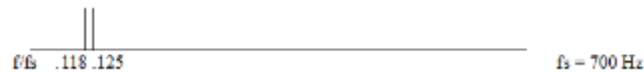
Figure 5 Difference in digital frequency between 82.4 Hz and 87.3 Hz if the sampling frequency is 700 Hz is .125 - .118 = .007
