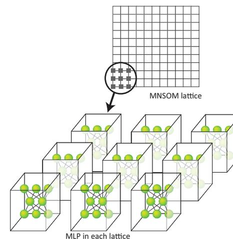
**Fig.3** Schematic diagram of MNSOM<sup>4)</sup>: The map consists from square lattice, and each vertex have network architecture.
