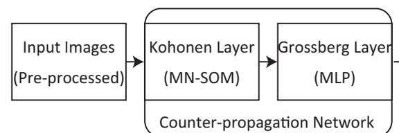
**Fig. 1** The schematic diagram of the Counter-propagation network. Input image is processed by the Kohonen layer with SOM type network, at first. Then, the output of the SOM is classified by the MLP corresponding to the Grossberg layer.
