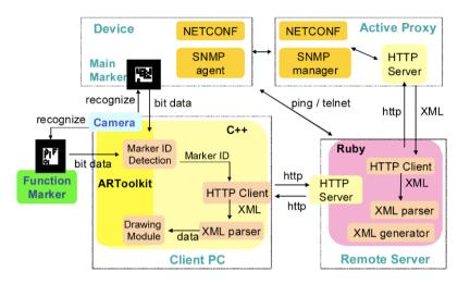
Fig. 1 TIARA architecture that contains 3 main components: Client, Server and Active Proxy
