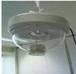
Fig.1 An omni-directional camera.
