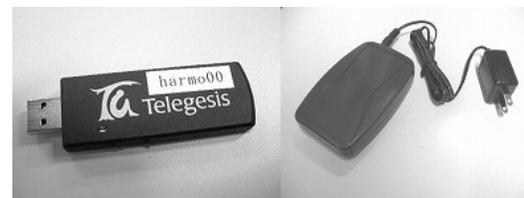
図 2 ZigBee modules: ETRX2USB (left), ETRX2 EAP-E(right)
