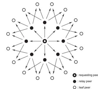
Fig.5 Pure flooding.
