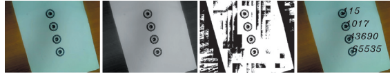
Fig. 6 The images from each phase in our system; input image, gray-scaling, binarization and detection (from L to R).
