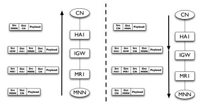
Fig. 4 Packet processing at IGW. Left: Outbound processing, Right: Inbound processing
