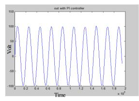
Fig.10 Simulated output with PI controller in case of no load
