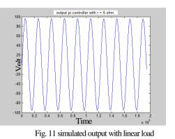
It can be seen that the load voltage has been reduced from 200 V to 196 V (98%). From sections 5.1 and 5.2, it can be seen using the PI controller improves the DC/AC inverter performance.
