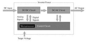
Fig.1 Block diagram of inverter power supply
