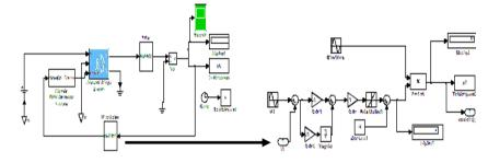
Fig.9a Closed loop Matlab model of DC/AC system
