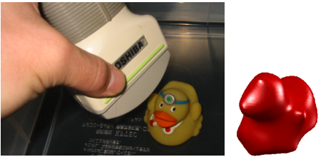
Fig. 13 Left: photograph of measuring a duck toy. Right: IP model of duck object
