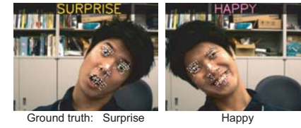
Fig.10 Some estimation results of facial poses and expressions with the fixed-pose dataset (In-plane rotation): The expression in the upper part of each image denotes the recognized result.
