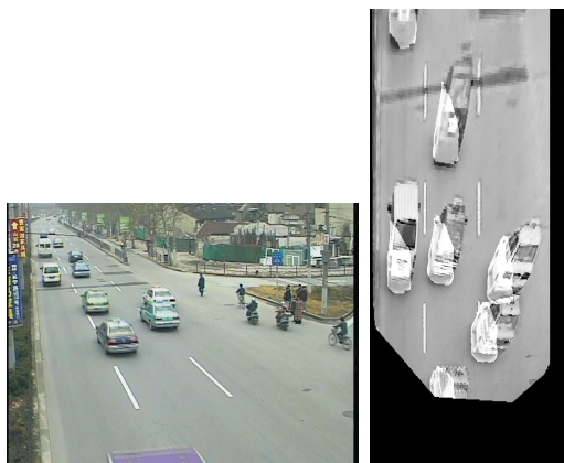
Fig. 13 Moderate to high volume traffic detection. Occlusion is seen in the left image. This occlusion is removed in the lower left image by the use of the IPM (Inverse Perspective Mapping) and the fusion of the images.
