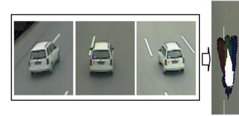
Fig. 5 Each camera in the system generates its own probability map. Each color in the image on the right is a region having a non-zero probability of representing the vehicle.
