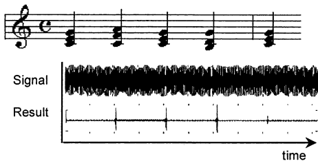
Fig.5 Simulation of Break Points Detection (Coif 5th, Detail3, T=0.05 [s])
