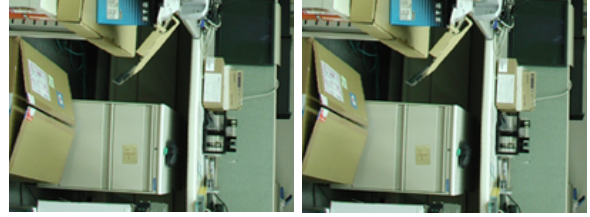
(b) After the viewing orientation is rotated 90 degrees, no stereo disparity is visible due to the lack of vertical parallax.
