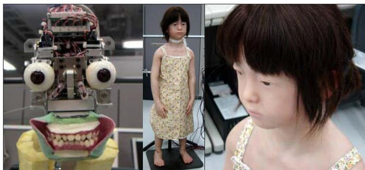
**Fig. 1** The android *Repliee R1* is a replica of a five-year-old Japanese girl. Her arms, neck, head, eyes, and eyelids are powered by DC motors fixed inside the robot. Her skin is made of silicone. In the photograph on the left, the android's skin, hair, and padding have been removed.
