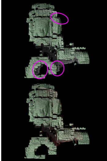
Fig. 31 Range data before and after the rectification method without images: the upper figure shows the original distorted shape by the FLRS (white) and the reference shape obtained by the Cyrax-2500 fixed on the ground(blue). The lower figure shows the recovered shape in the lower figure (pink) fitted onto the correct one.
