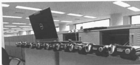
Figure 5. Ten webcams connected to a laptop via a USB hub.
