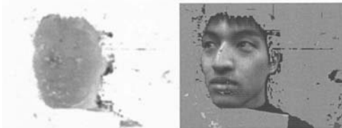
Figure 7. Real-time depth map computation from four webcams.
