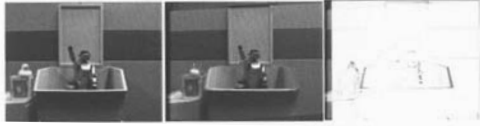
Figure 4. Left: real view. Center: computed view. The virtual camera is placed between two adjacent input cameras. Right: difference between real and computed view.
