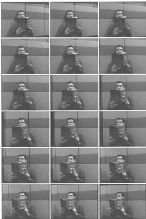
Figure 6. Each new view is computed on-line with a laptop using 4 cameras selected between 10. The scene was discretized with 60 planes and this method reaches 15 fps.
