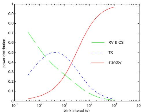
Fig. 5 Power consumption distribution in non-p CSMA system
