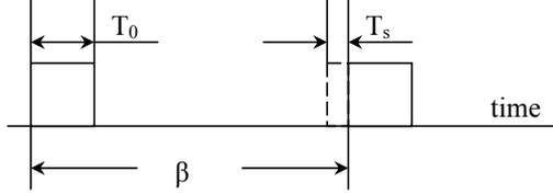
Fig. 1 timing of tag blinks
