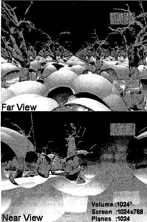
Fig.6: The sample scene consists of a repeatedly rendered 1024^3 dataset and contains numerous complex shapes in order to provide an accurate measurement.
