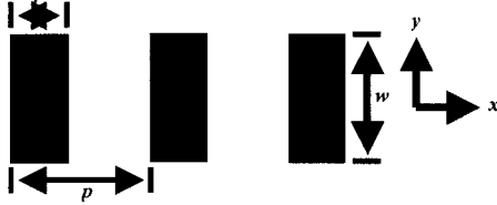
Fig.3. Layered Structure. Layer thickness t = 94\text{nm} , periodicity p = 235\text{nm} , width w = 329\text{nm} . There are 9 layers (not all shown). Dark area is dielectric material of refractive index n = 1.6 .
