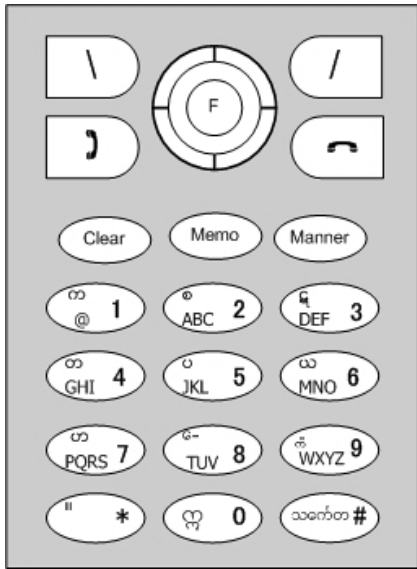
Fig.3. Multitap keypad layout
