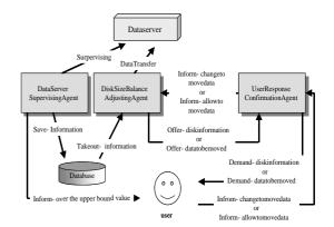
Figure 1: Structure of the parallel I/O control agent
