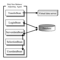
Figure 3: Implementation of the Disk Size Balance Adjusting Agent
