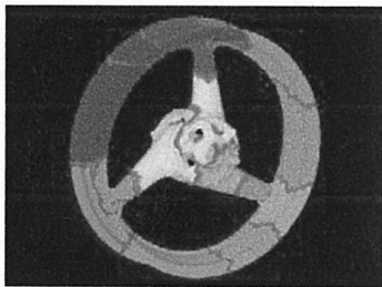
Figure 2 Model of motor cycle wheel partitioned into 16 domains
