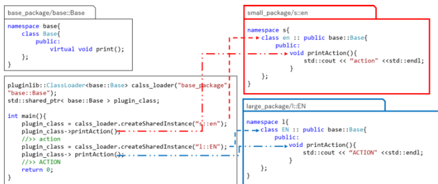
Fig. 3 Example of change the main class by using pluginlib
