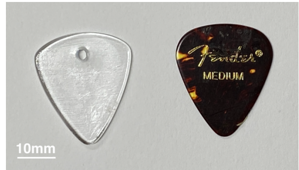
図3 ピック: シリカガラス製 (左) セルロイド製 (右) Figure 3 Plectrum: made of silica glass (left), celluloid (right)
