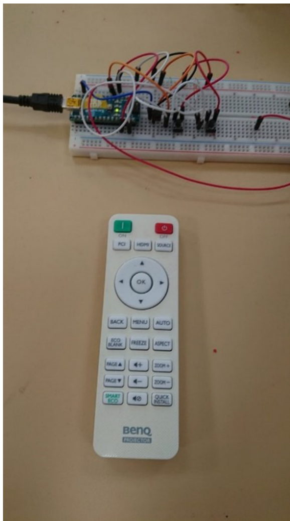
Fig. 8 Receiving the IR command using the IR transceiver.
