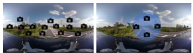
Fig. 5 Virtual camera generation area. Left is in initialization, right is in tracking.
