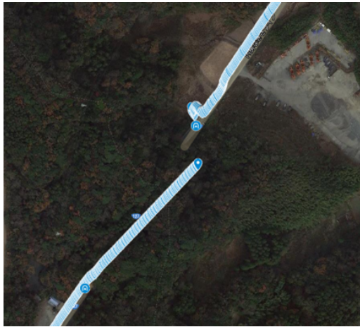
Fig. 2 Wrong GPS information in tunnel.
