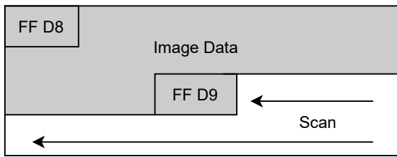
Fig. 9 Illustration of scanning to detect the end of image file
