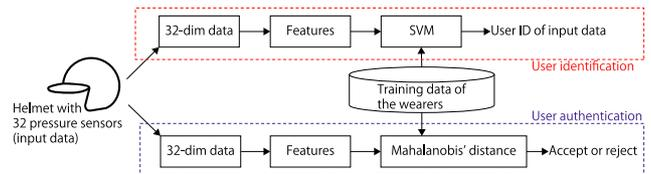
Fig. 1 Process of user identification and authentication.
