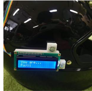
Fig. 8 LCD display to show name.
