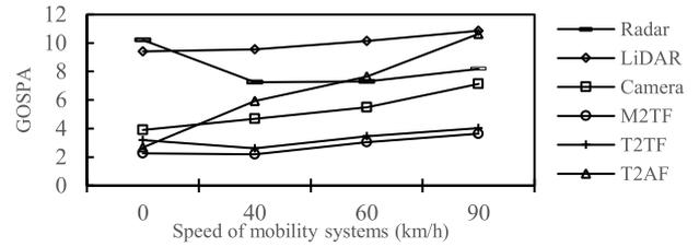
**Fig. 15** GOSPA performance evaluation for tracking and fusion at different speeds in normal case.
