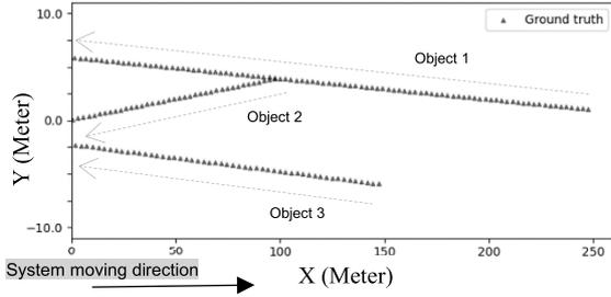
**Fig. 12** The visualization of the trajectories of three objects under moving system with the speed 90 km/h.
