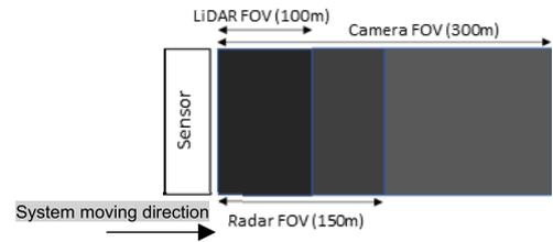
**Fig. 11** The illustration of FOV for sensors in simulation.
