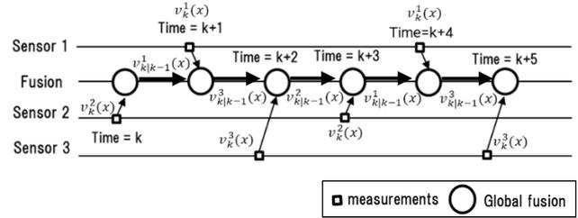
**Fig. 5** The measurement management of measurement-to-track fusion with GMPHD integration.
