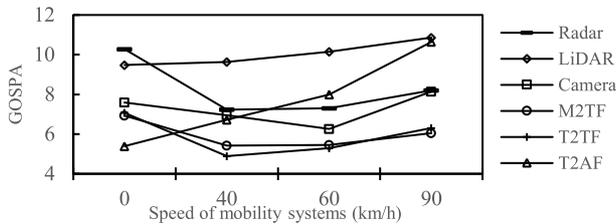
**Fig. 25** GOSPA performance evaluation for tracking and fusion at different speeds in abnormal case with camera detection rate 50%.
