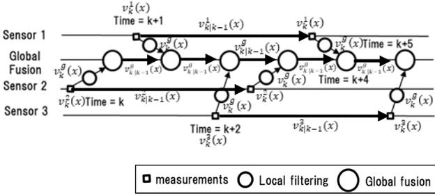
Fig. 7 The measurement management of track-to-track fusion with GM-PHD integration.
