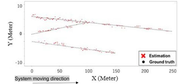
**Fig. 27** Fusion result with M2TF architecture for mobility system at 90 km/h in abnormal case with camera detection 0.5.
