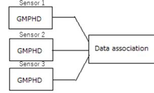
Fig. 8 The structure of track-to-association fusion with GMPHD integration.
