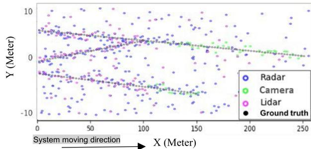
**Fig. 19** The simulation measurement for mobility system at 90 km/h in abnormal case with camera detection 0.75.
