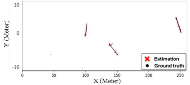
**Fig. 21** Fusion result with T2AF architecture for mobility system at 0 km/h in the case with camera detection rate 0.75.
