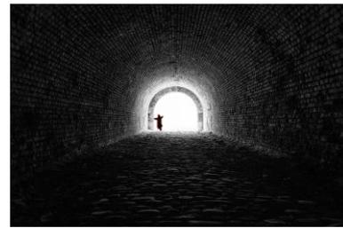
**Fig. 29** Unrecognizable object near the tunnel exit due to the backlight effect in exemplary optical sensor's image.
