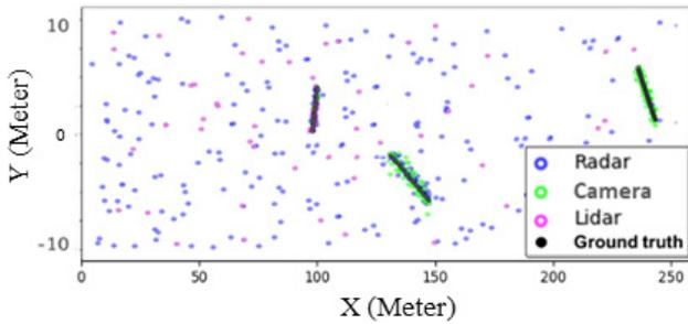
**Fig. 13** The simulation measurements from all sensors at 0 km/h in normal case.
