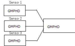
**Fig. 6** The structure of track-to-track fusion with GMPHD integration.
