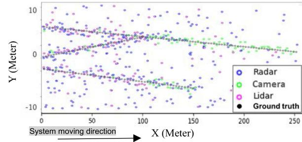
**Fig. 14** The simulation measurements from all sensors at 90 km/h in normal case.
