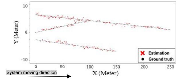
**Fig. 22** Fusion result with M2TF architecture for mobility system at 90 km/h in the case with camera detection rate 0.75.
