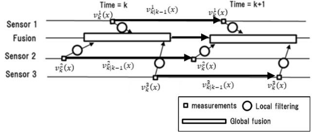
Fig. 9 The measurement management of track-to-association fusion with GMPHD integration.
