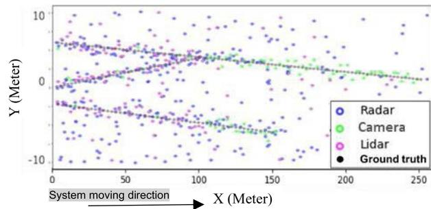
**Fig. 24** The simulation measurement for mobility system at 90 km/h in abnormal case with camera detection rate 0.5.
