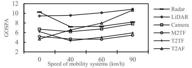
**Fig. 20** GOSPA performance evaluation for tracking and fusion at different speeds in abnormal case with camera detection rate 75%.
