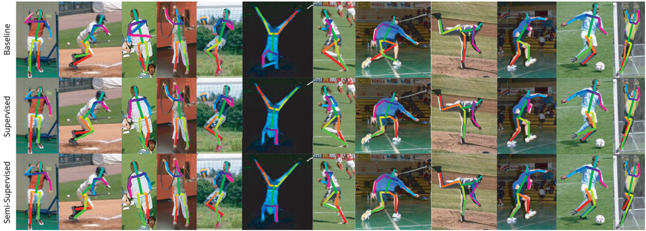
Fig. 10 Examples of pose estimation obtained by the baseline method [30], the supervised and semi-supervised versions of MirrorNet. Anatomically implausible poses were corrected by the MirrorNet architecture.
