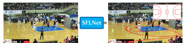
Fig. 1 Our single shot regressor, SFLNet , directly regresses a set of parameters that corresponds the metric model of a sports field (shown in top right on the right image) to the court seen in an input frame. Best viewed in color.
