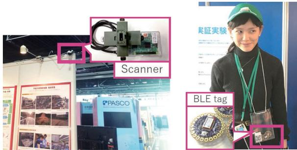
(a) Scanner placement. Most scanners were placed at the top of partitions. (b) Experiment subject with BLE tag in GEXPO2016.
