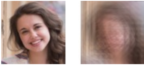
Figure 1. (Left) Normal image, (Right) Multi-pinhole image
