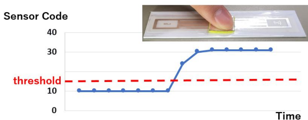
Fig. 4 Transition of Sensor Code in pressure monitoring
