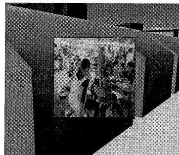
Figure 12: A replaying video plane positioned in the center of a window because of synchronization of a virtual camera and a real camera.
